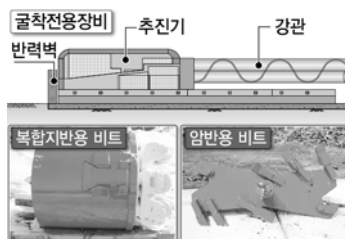
Fig. 6 Machine excavation with exclusive equipment
