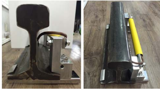
Fig. 3 Prototype of rail-mounted displacement sensor
