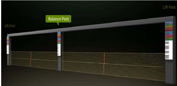
Fig. 2 Configuration of RPSD Structure
