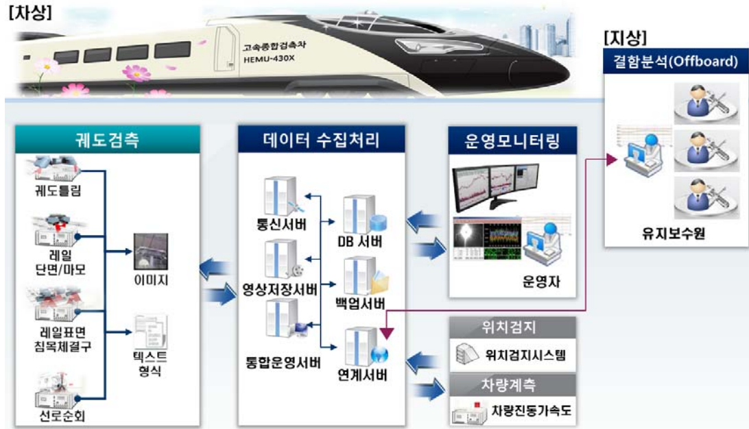
Fig. 1 The concept of High Speed Track Measurement System
