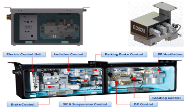
Fig. 1 In Miniature Function(top) and Extended Function(bottom) Air Brake Control Device
