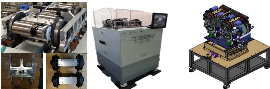
Fig. 6 1/5 small scale roller rig to evaluate individual wheel torque control strategy
