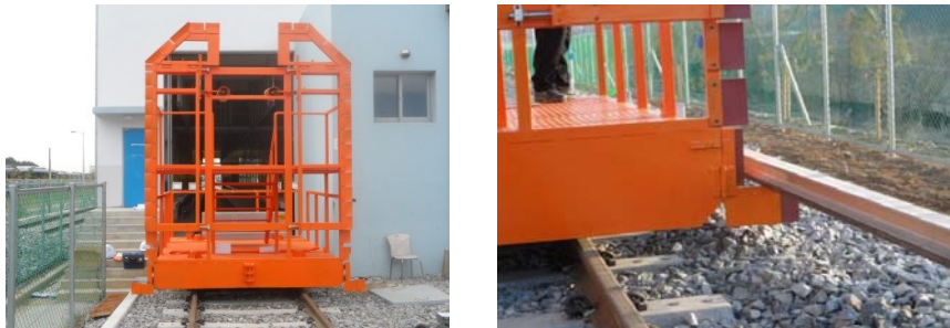
Fig. 2 Measurement Gear of the Construction Gauge
