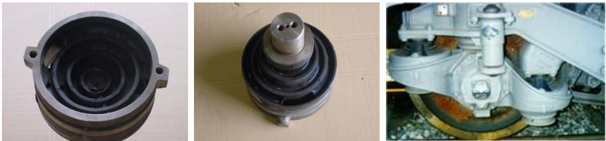
Fig. 2 Conical rubber spring for railway vehicle
