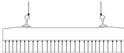
Fig. 1 Results of structural analysis for wide sleeper on asphalt track in high-speed railroad
