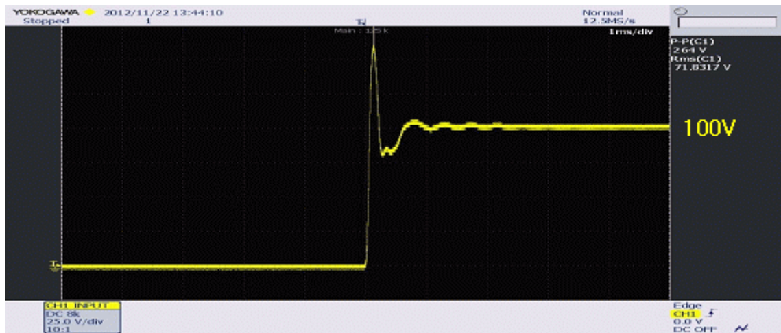
Fig.5 Measures the Peak voltage across the capacitor
