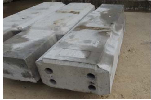
(b) Wide sleeper of non-installed reinforcing bar
