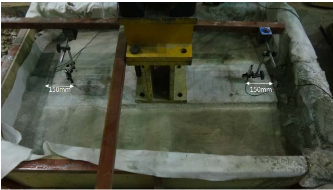
Fig. 4 Measuring instrument and under loading part
