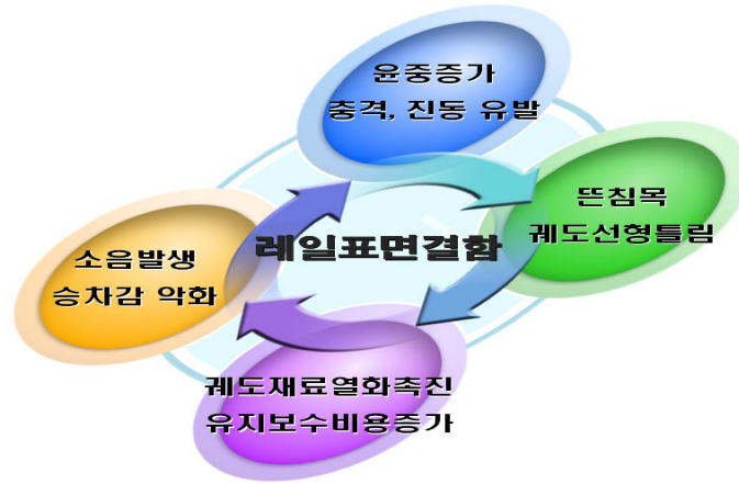
Fig. 3 Influence of rail surface defect
