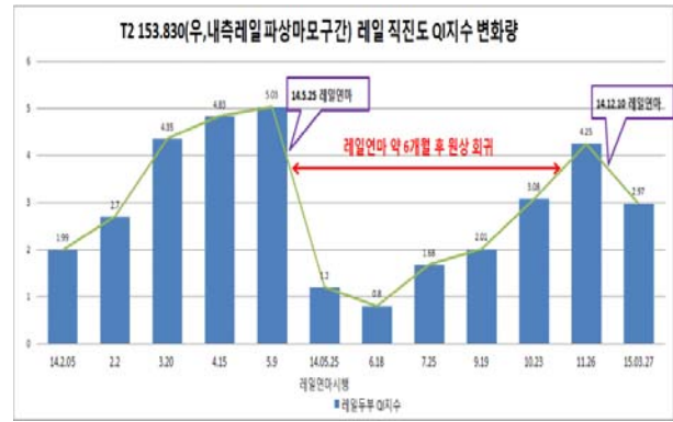
Fig.7 The calculation of rail grinding period
