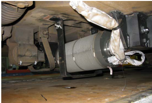
Fig. 2 Actuator installed under the bogie
