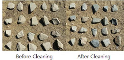
Fig. 4 The Result of Gravel Cleaning
