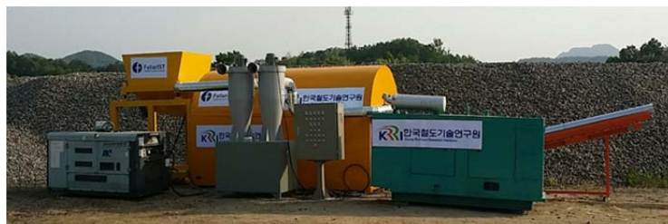
Fig. 3 The Installed Gravel Cleaning Machine
