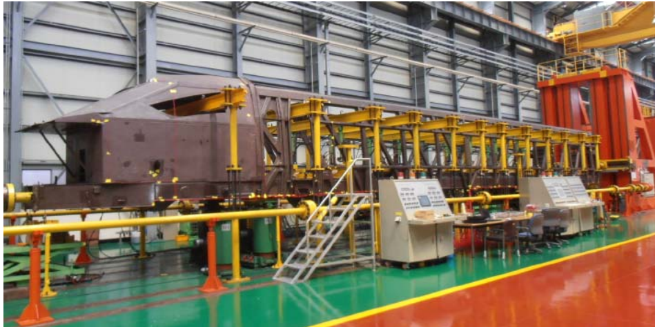
Fig. 1 JIG Setting for Power Car Body Load testing
