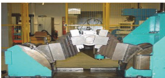
Fig. 3 Installed chevron rubber spring for measurement
