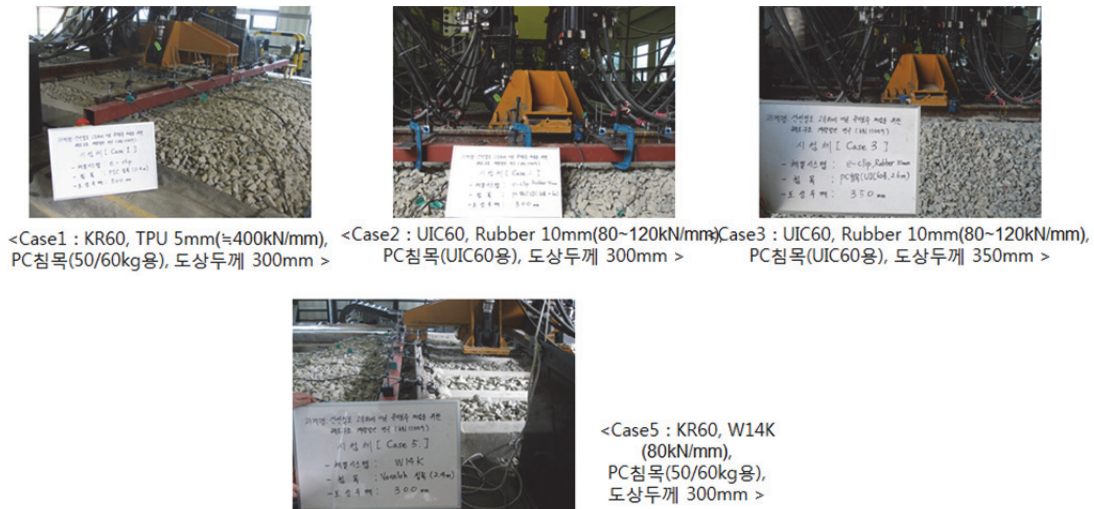
Fig. 5 Dynamic tests of full-scale specimens
