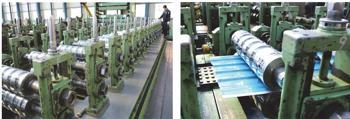
Fig. 3 Roll forming machine and roll forming of a LDSS roof panel
